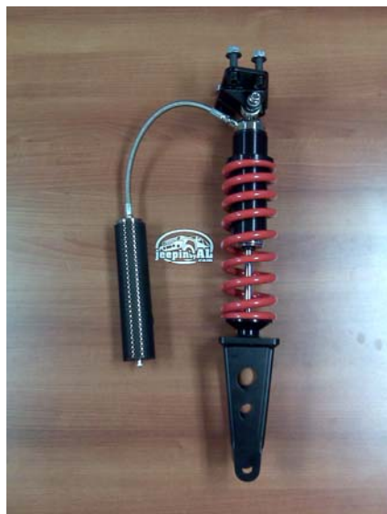
Front struts for the Jeep Liberty w/ remote reservoir
