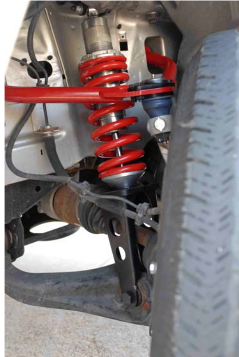
Struts installed in 2008 KK w/ JBA Upper Control Arms
