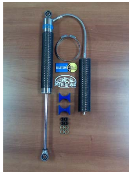
Rear shock w/ remote reservoir for the Jeep Liberty
